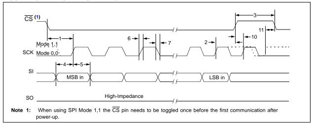
FIGURE 1-6: SPI OUTPUT TIMING
