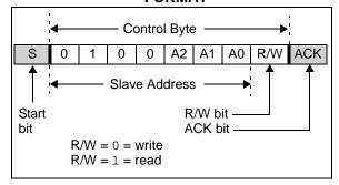
FIGURE 3-5: SPI CONTROL BYTE FORMAT
