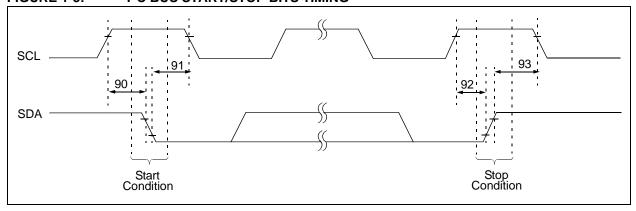
FIGURE 1-4: I<sup>2</sup>C BUS DATA TIMING
